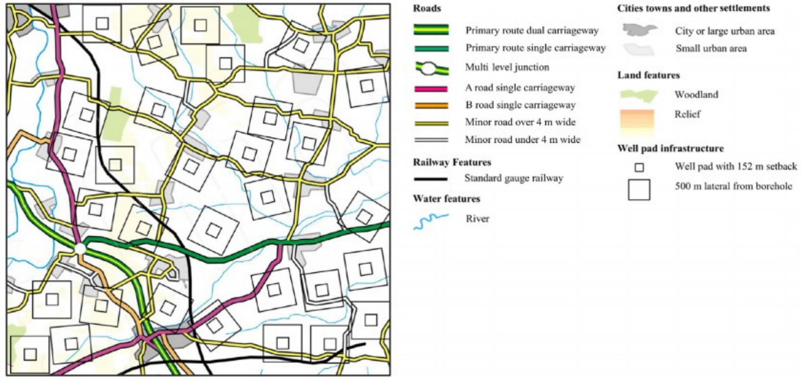
Figure 4 Illustrative example of well pad density estimation from Clancy et al (2017, Fig 3 in original document). Inner squares show recommended 152m setback, outer squares the potential extent of 500m lateral drilling. Block size is 100km 2 with 31 well pads in this example.
